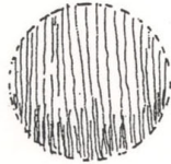
Parallel Line Line up side by side in parallel fashion [Use for flat smooth obj and to show distance]
