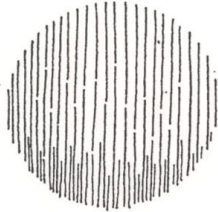
Parallel Line Line up side by side in parallel fashion [Use for flat smooth obj and to show distance]
